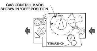
gas, including near the floor. If you smell gas, STOP! Follow "B" in the safety information above. If you don't smell gas, go to the next step. 8. Turn gas control knob counterclockwise 🛩
